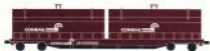
Coil steel flat / 12" symbols with 5" logotypes. Coil stack to receive 26" symbols with 10" logotypes.
