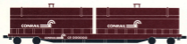
Coil steel flat / 1'3" symbols with 5" logotypes. Coil covers to receive 2'6" symbols with 1'0" logotypes.
